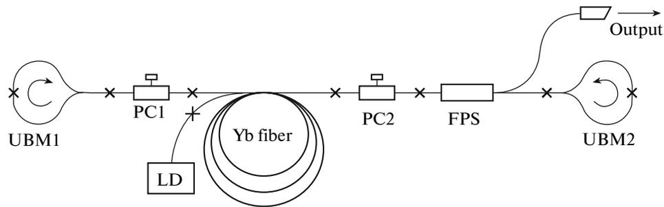
**Fig. 5.** Scheme of the proposed ultrashort-pulse ytterbium laser with the linear cavity and two ultrabroadband fiber reflectors: LD pumping laser diode, UBM1 and UBM2 ultrabroadband fiber mirrors, PC1 and PC2 fiber polarization controllers, and FPS fiber polarization splitter.
